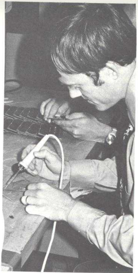
Bob Ridings solders a printed circuit card for use in the SPEC system.
