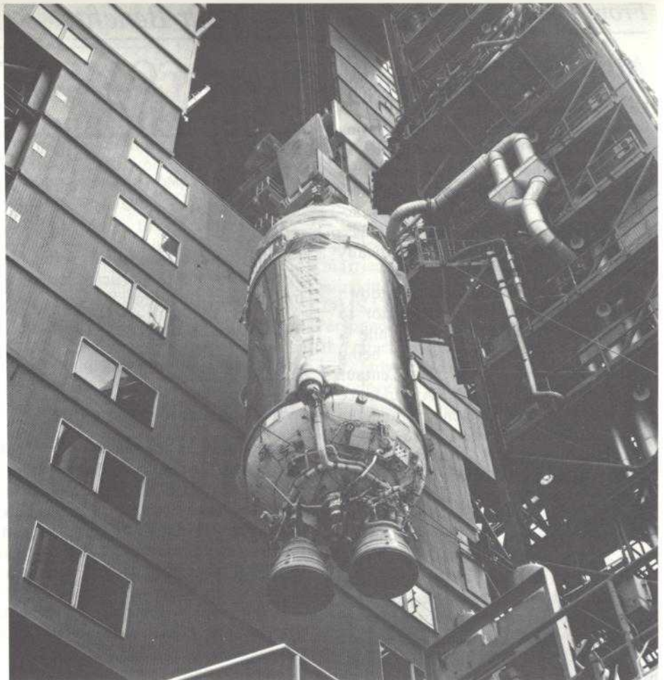
The Centaur stage as it moves into place to be mated to the Atlas booster.
