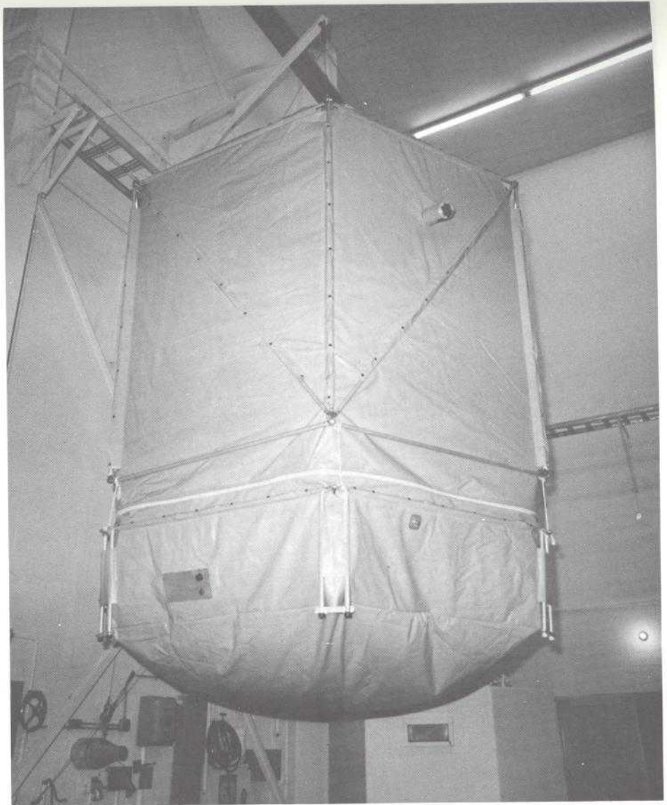
A huge protective cover is used to protect the assembled spacecraft during transportation from the test facilities at Hangar AM to the launch pad. The bag is also used to cover the spacecraft in earlier tests to check valves and tubing for hydrazine leaks.
