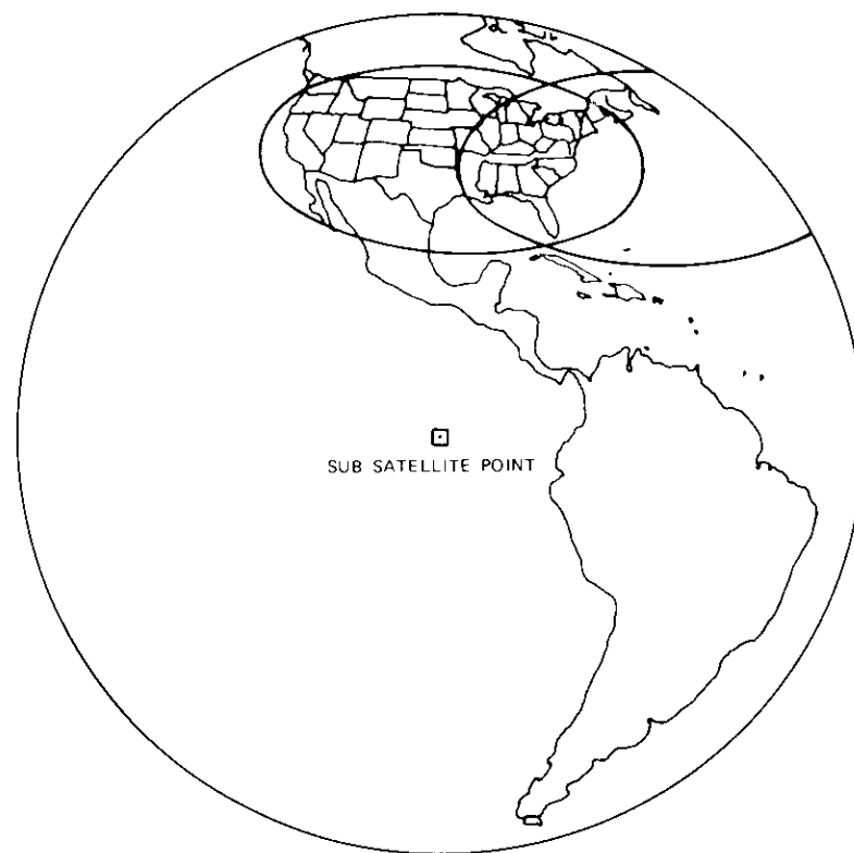
Figure 2. Spacecraft Receive Antenna Coverage
