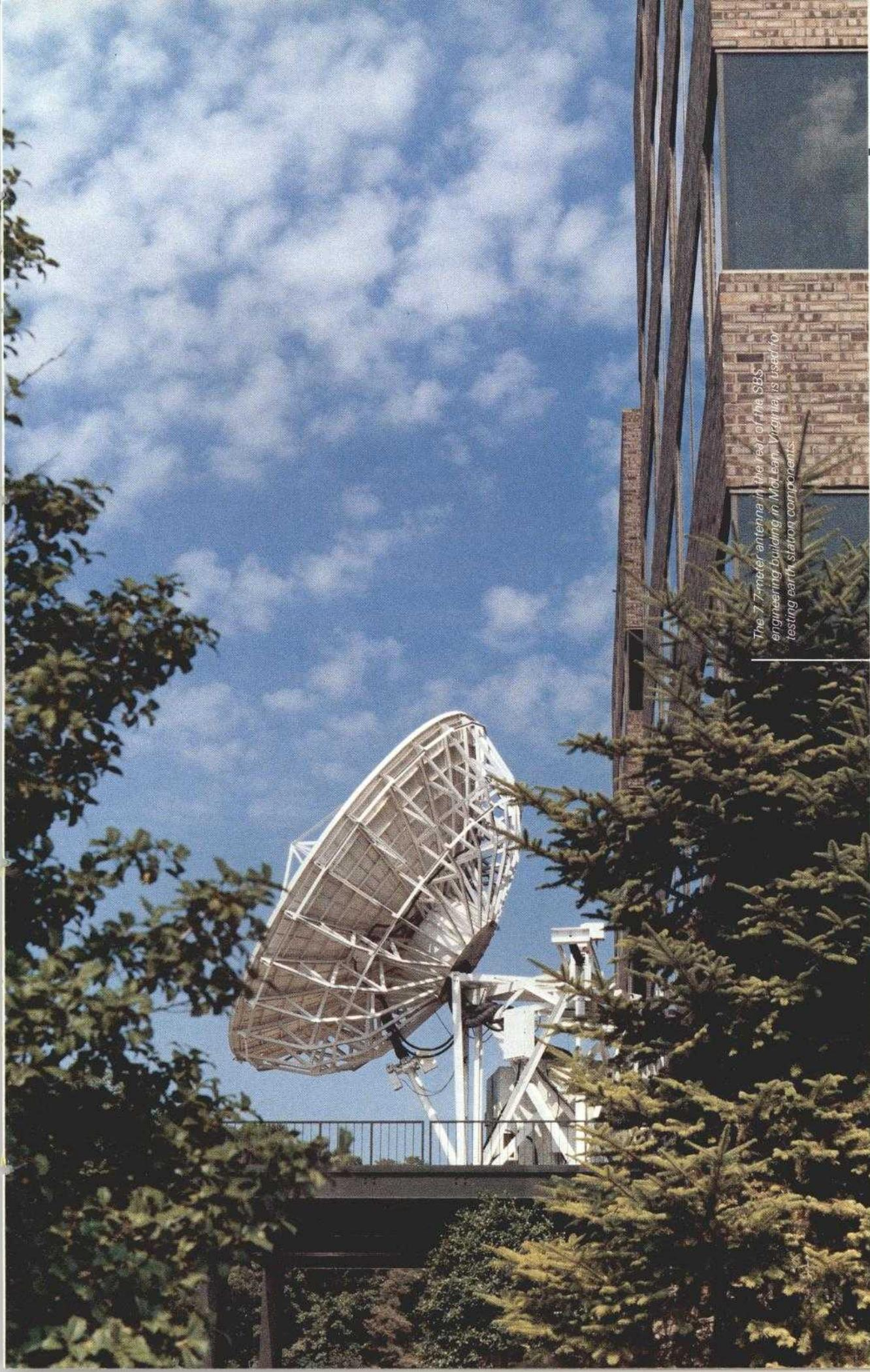
*The 7.7-meter antenna in the rear of the SBS engineering building in Mallean, Virginia, is used for testing earth station components.*
